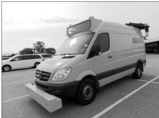
Figure 9: Automatic Road Analyzer Vehicle
