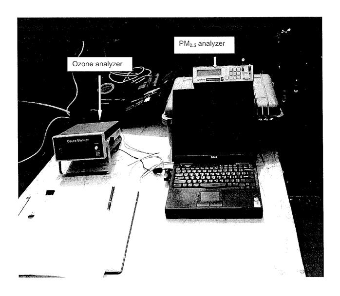
Figure B-1: Ozone and PM<sub>2.5</sub> Analyzers
